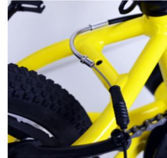
1. Disconnect the rear brake to allow better clearance
