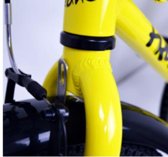
1. Place the mudguard between the fork legs, ensure that one metal tab is placed in front of the fork and one metal tab behind the fork.
