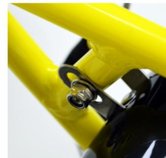
4. On the underside add the second metal washer under the seat stay.
