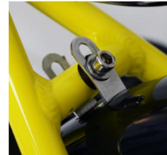
6. Adjust the mudguard up and down until sufficient tyre clearance is achieved.
