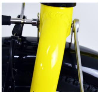
5. Tighten up the mudguard to secure it with the spanner and allen key to 4Nm.
