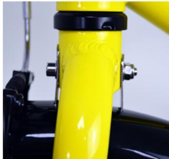
2. Insert the bolt with a metal washer on either side of the adjustable bracket, and lightly tighten the nut.
