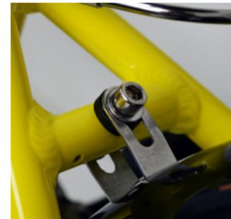
3. Add the first metal washer and bolt into the assembly.
