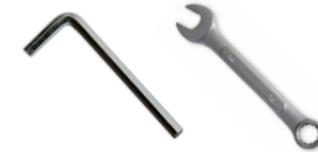
5. Lightly Install the bolt using a 10mm spanner and a 4mm allen key.
