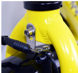
4. Adjust the mudguard up and down until sufficient tyre clearance is achieved.
