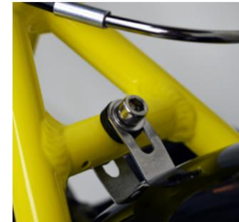
7. Tighten up the mudguard to secure it with the spanner and allen key to 4Nm.
