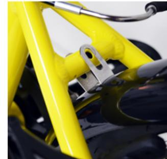
2. Insert the mudguard. Slide the adjustable bracket inline with the seat stay bridge
