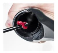
19. Grease the outer stanchion bushes and foam rings using a dowel rod.
