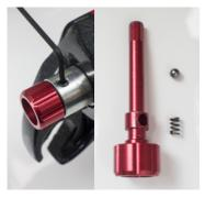
4. Frog 69/72 MTB Only. Remove Rebound control knob using 1.5mm Allen key. N.B Under the grub screw is a small bearing and spring. Take care not to lose these parts.
