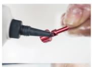
23. Re-assemble Rebound control knob. Apply a small amount of grease to hold spring and bearing in place. Insert back into bolt and tighten the grub screw in place using 1.5mm Allen key.
