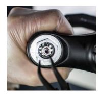
6. Remove circlip.
