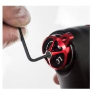
Remove red lockout adjustment lever.
