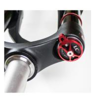
1. Set fork in locked out position and remove from frame.
