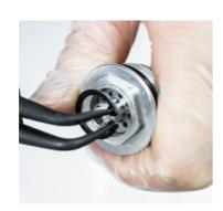
5. Re-fit circlip, locating correctly into the recess.
