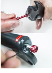
24. Re-fit red lockout adjustment lever. The fork should be in locked out position with cap in the appropriate position.
