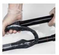
20. Slide the inner and outer stanchions back together. N.B. The fork brace is on the back of the outer stanchions!
