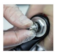
4. Relocate the lockout control rod.
