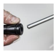
14. Remove rubber top out buffer from inner air rod.
