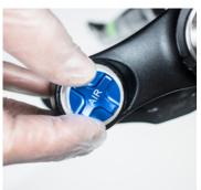
2. Remove blue air valve dust cap.
