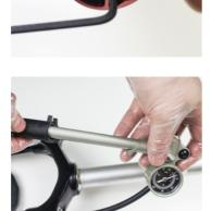
25. Pressurise the fork using a shock pump to approx. 50psi. (0271)
