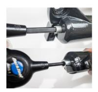
9. Undo lower stanchion bottom bolts. 6mm/5mm. N.B Compress forks & make an initial sharp twist to break thread seal.
