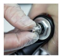
7. Lift out lockout control rod.
