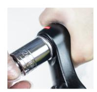
8. Tighten using 22mm socket. 18Nm
