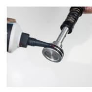
9. Grease air valve piston assembly.
