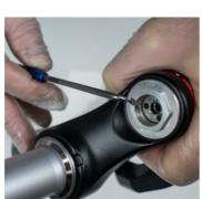
8. Remove 3 Ball bearings and springs using a magnetic pick.
