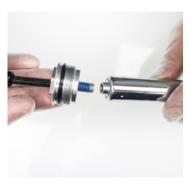
Attach alloy lockout top cap to oil cartridge using the lockout assembly bolt.
