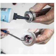
2. Add a small amount of grease to each of the 3 holes in the lockout assembly bolt.
