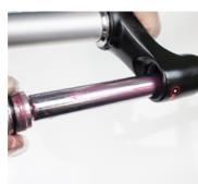
7. Relocate cartridge into the lockout side of the Inner stanchions.
