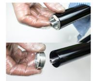
15. Slide inner air rod up and use a 24mm socket to undo and remove alloy bottom air cap. Then slide out air valve piston assembly.
