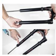
17. Slide NEW wiper seals & soaked foam rings onto the Inner stanchion legs and lightly grease.
