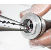
3. Carefully relocate the springs and ball bearings.
