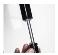
13. Pull out inner air rod and fit rubber top out buffer.
