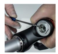
8. Remove 3 Ball bearings and springs using a magnetic pick.
