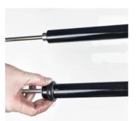
17. Slide NEW wiper seals & soaked foam rings onto the Inner Stanchion legs and lightly grease.
