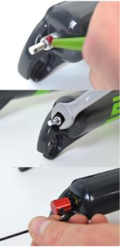
23. Re-assemble rebound control knob. Apply a small amount of grease to the rebound thread. Reinstall the spacer and nut with a 10mm spanner. Install the switch with a 2mm allen key.
