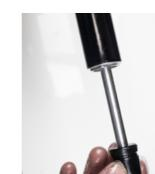
13. Pull out Inner air rod and fit rubber top out buffer.
