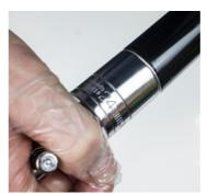
12. Re-tighten in the inner stanchions. 18Nm
