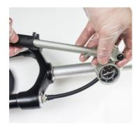
25. Pressurise the fork using a shock pump to approx. 50psi. (0271)
