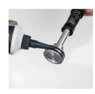
9. Grease air valve piston assembly.
