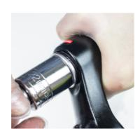
8. Tighten using 22mm socket. 18Nm
