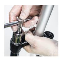
16. Unscrew alloy air valve seal top cap using 24mm socket.
