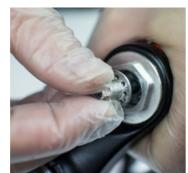
7. Lift out lockout control rod.
