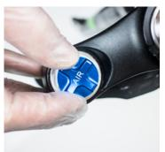
2. Remove blue air valve dust cap.
