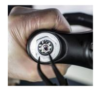
6. Remove circlip.
