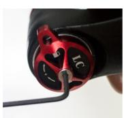
24. Re-fit red lockout adjustment lever. The fork should be in locked out position with cap in the appropriate position.
