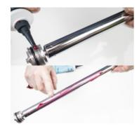
6. Lightly grease lockout top cap thread and outer surface of the oil cartridge.
