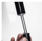
7. Relocate cartridge into the lockout side of the Inner stanchions.
