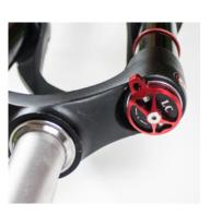
1. Set fork in locked out position and remove from frame.
